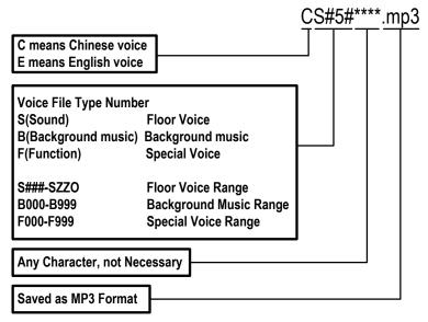
The last 3 bits in 'S#5#' (#5#) are corresponding to 3 bits setting display. The setting range as follows:
