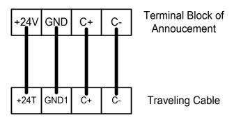
Figure 4 Wiring Diagram
